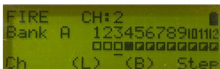
**Note:** If button 1-12 is held down a continuous pulse is sent to the receivers until the button is released.
