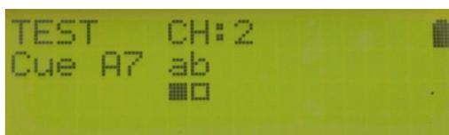
In this example Cue A7 has got continuity on module with ID “a”, but no continuity on module with ID “b”.
